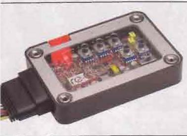
■ **RE-Q** is designed to adjust the bass and treble signal of virtually any stock head unit to get the best possible response and sound when adding subwoofers, amplifiers and auxiliary speakers to a primarily stock audio system. Now you can obtain the bass you want without having to ditch your OEM head unit and factory audio controls. **\$150**
